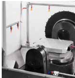
Wash down system
